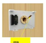
(7) Buckle connectors indoor bracket and outdoor device(as FPCB containing dedicated circuit,pls attention its intensity when fastening connector,to avoid too much force to demage FPCB or connectors)
